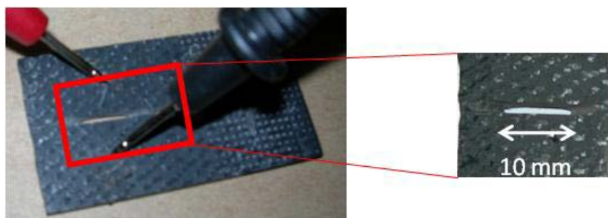
Figure S2. Electrically-induced heating in a nano-engineered composite plate with a 10 mm long through-crack using simple electrical probes; thermographs shown in figure 1(b).
