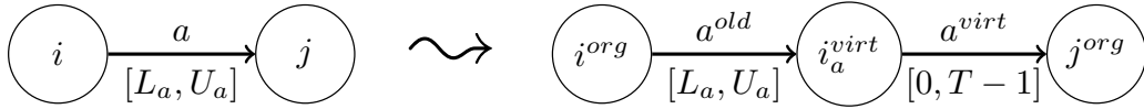
■ Figure 2 Extending an activity a = (i, j) \in A with span \Delta_a = [L_a, U_a] to two activities a^{\text{old}} = (i^{\text{org}}, i_a^{\text{virt}}) \in \mathcal{A}^{\text{old}} with span \Delta_a^{\text{old}} = [L_a^{\text{old}}, U_a^{\text{old}}] := [L_a, U_a] and a^{\text{virt}} = (i_a^{\text{virt}}, j^{\text{org}}) with span \Delta_a^{\text{virt}} := [0, T - 1] .
