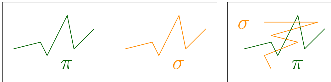
■ Figure 1 Curves with similar shape but large DTW distance (left) and different shape but small DTW distance (right).
