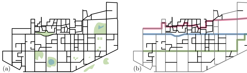
■ Figure 1 (a) A road network can be represented as a graph G . (b) Edges in G can be weighted, e.g. depending on whether traffic flows fast (grey) or slow (black). Under the shortest path metric, the Fréchet distance between blue and green may be smaller than the distance between red and black; even though under the Euclidean metric, the red-black Fréchet distance is smaller.
