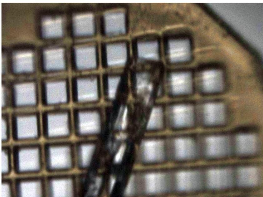
**Supplementary Figure 1.** Trichovirin I-4A crystal mounted on a micromesh support for data collection. The mesh size is 25 $\mu$ m.
