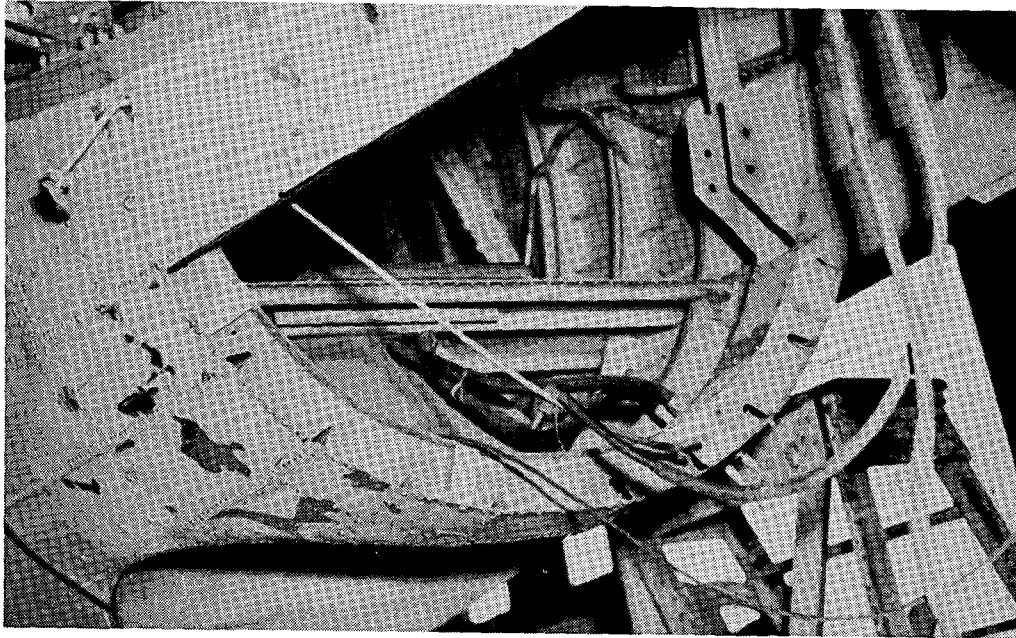
3. Detail of the inferior door of inspection and of the cone reactor mounting.
