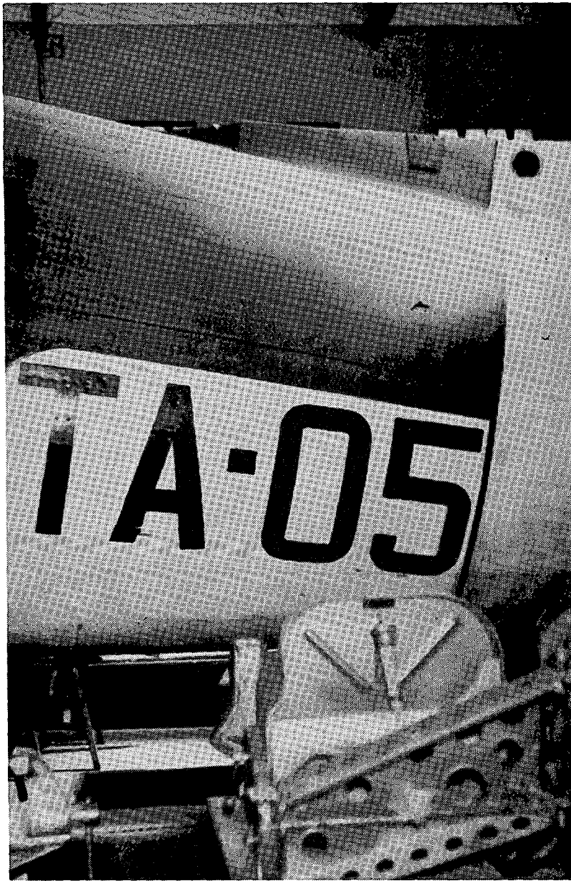
1, View of the fuselage-cone union part. In the superior part, the driven back reactor's air inlet may be seen.
