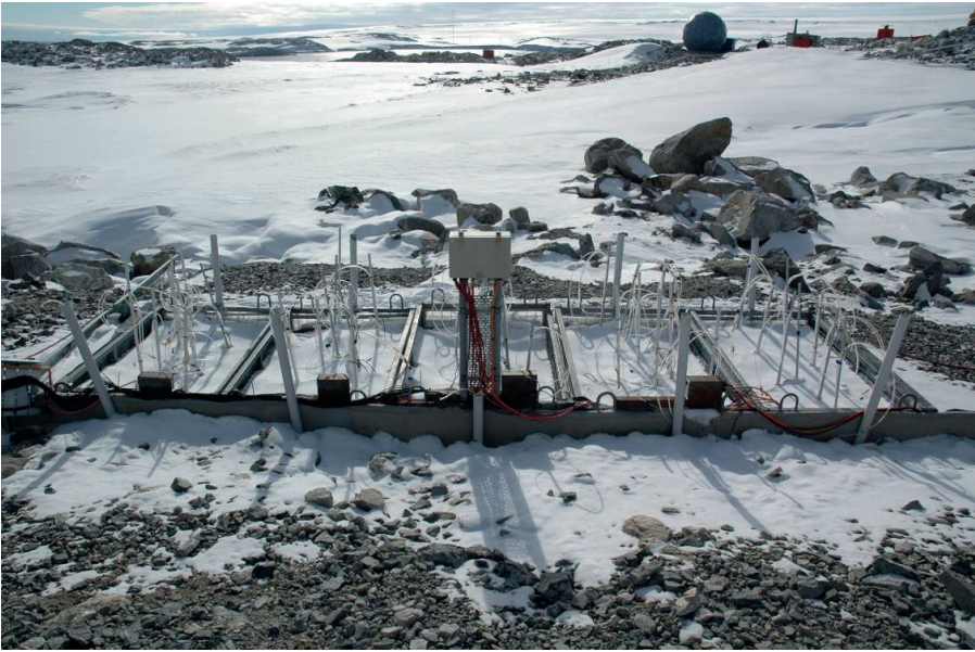
Photo 7: Heavily instrumented gate used for research purposes and trialling a variety of granular media.
