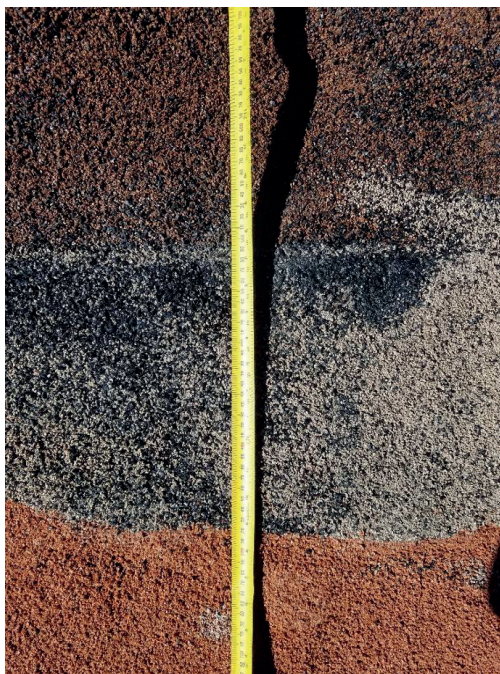
Photo 5: Top view of sequenced granular media in PRB. In this instance, showing zeolite (orange), granular activated carbon (black) and nutrient enriched zeolite (white). Water flow is from bottom of picture towards the top.
