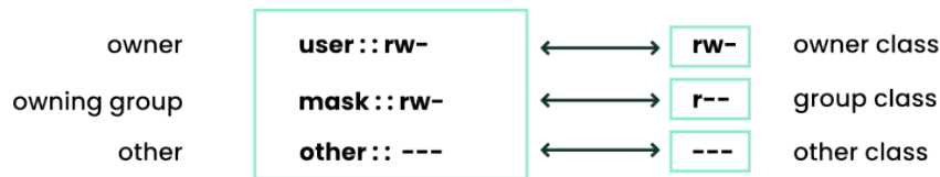
FIGURE 19.1: MINIMUM ACL: ACL ENTRIES COMPARED TO PERMISSION BITS
