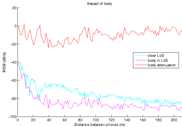
Fig. 5. LoS measurements w/ and w/o body.
