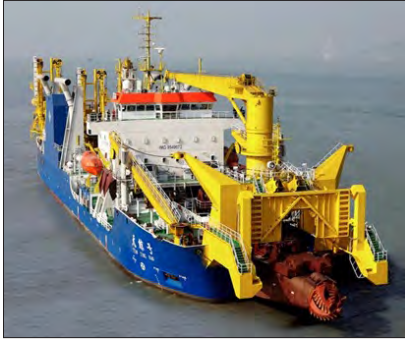
Figure 15: Tian Jing Hao, Cutter-Suction Dredge (Annex 858)
