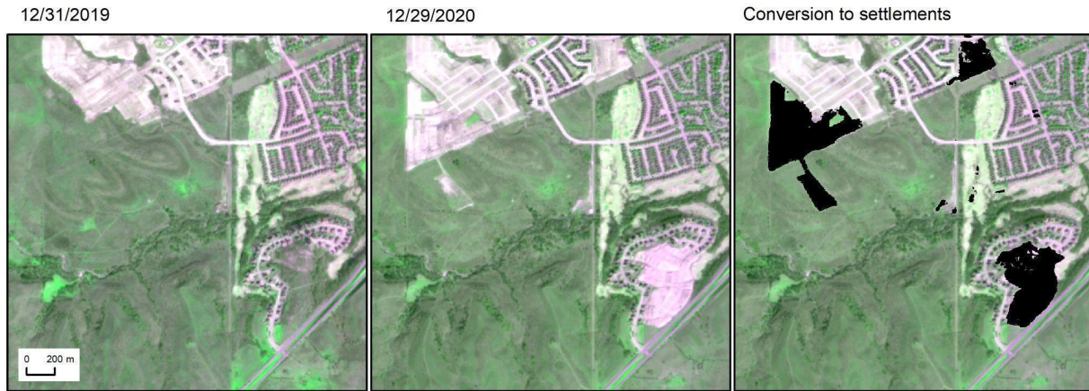
Figure 3.4: Examples of vegetation disturbances that are captured in the DIST product suite (images from PlanetScope, false color composite of Red-NIR [near-infrared]-Green). Here, vegetation is characterized by shades of green and gray, and bare ground by shades of pink. In the final column, black represents areas of conversion. Top row: Vegetation conversion to mining in Indiana. Bottom row: Vegetation conversion to urban development in Dallas, TX. From RD2.
