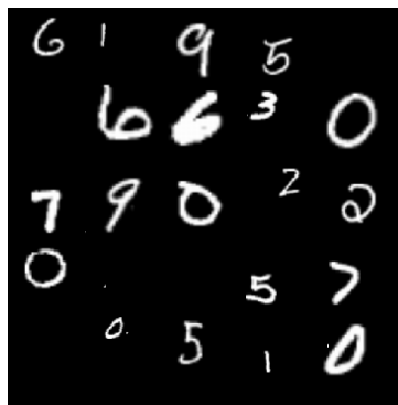
Fig. 20: Multiple object classification consists of mapping an image to a multiset of class labels. In this example, any ordering of the digits \{0, 0, 0, 0, 0, 1, 1, 2, 2, 3, 5, 5, 5, 6, 6, 6, 6, 7, 7, 9, 9\} is a valid labeling.
