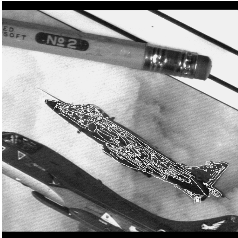
Figure 8.12 The Sea Harrier test input with the retrieved model overlaid on it. The recovered transformation (rotation, translation and scaling) was based solely on the basis pair, and not on a best least-squares match of all corresponding feature pairs.
