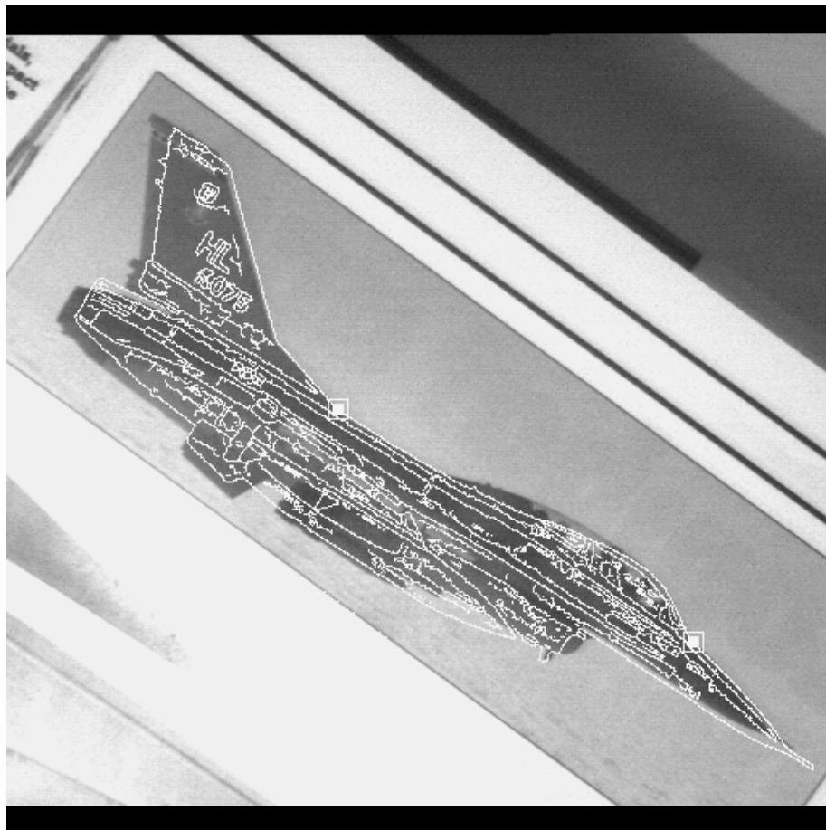
Figure 8.10 The F16 test input with the retrieved model overlaid on it. The recovered transformation (rotation, translation and scaling) was based solely on the basis pair, and not on a best least-squares match of all corresponding feature pairs.
