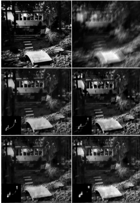
Figure 5.4: Recovery of a 27 \times 27 kernel. Top-left: original; top-right: blurred; middle-left: deblurred with ground truth kernel; middle-right: deblurred with our estimated kernel; bottom-left: deblurred with kernel of [55]; bottom-right: deblurred with kernel of [142]. Corresponding kernels are shown as insets at the bottom left of each image.
