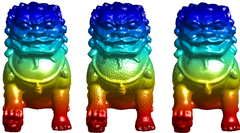
Figure 7.12: Example of mesh smoothing using an inhomogenous Laplacian based on an inverse distance measure between vertices. Left: original mesh; Middle: noisy mesh; Right: denoised mesh with our solver with smoothing parameter t = 0.1 .
