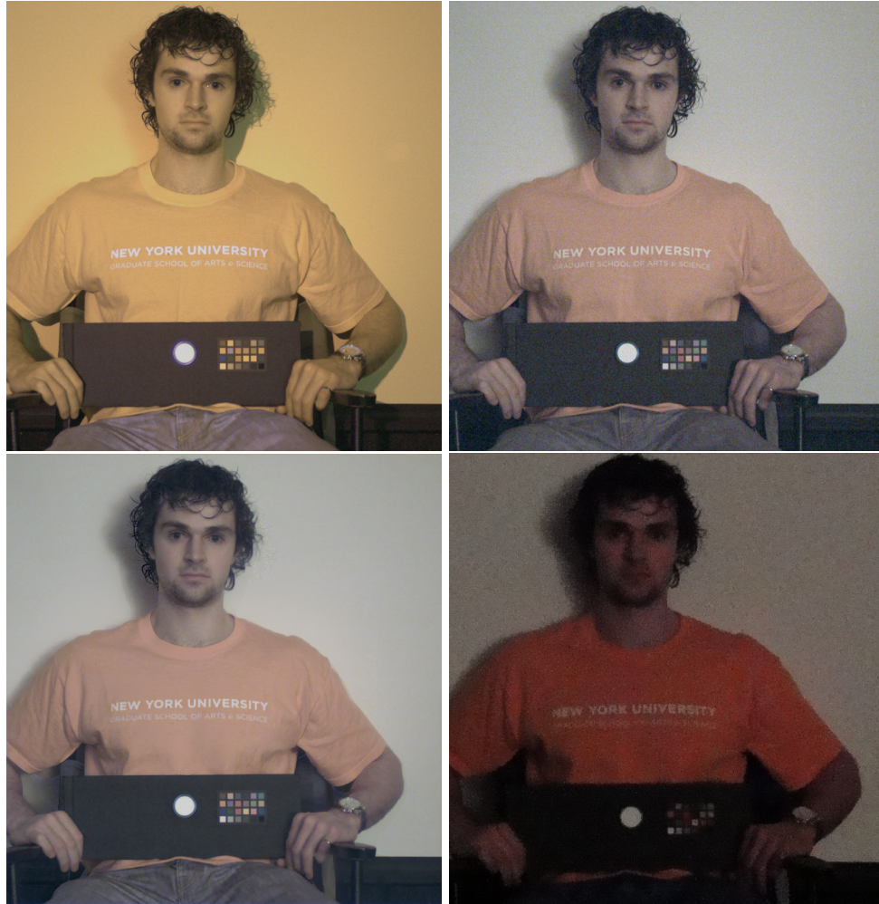
Figure 3.12: Denoising at extremely low light levels (0.7 Lux). Top-left: UV/IR Flash shot; Top-right: Noisy Ambient; Bottom-left: Our reconstruction; Bottom-right: Image taken from Sony NightShot camera.
