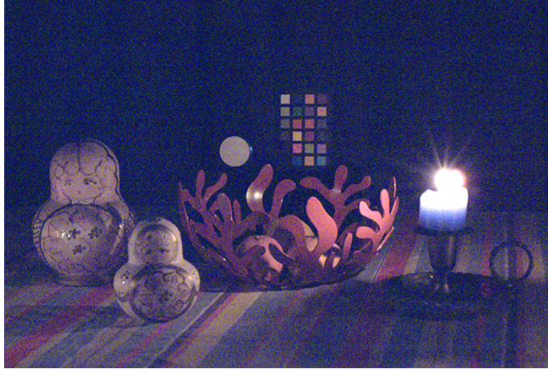
Figure 1.1: An image taken with illumination from a candlelight. High noise levels are clearly visible, especially in the blue channel. Even state-of-the-art denoising methods do not perform well at such low signal-to-noise ratios.
