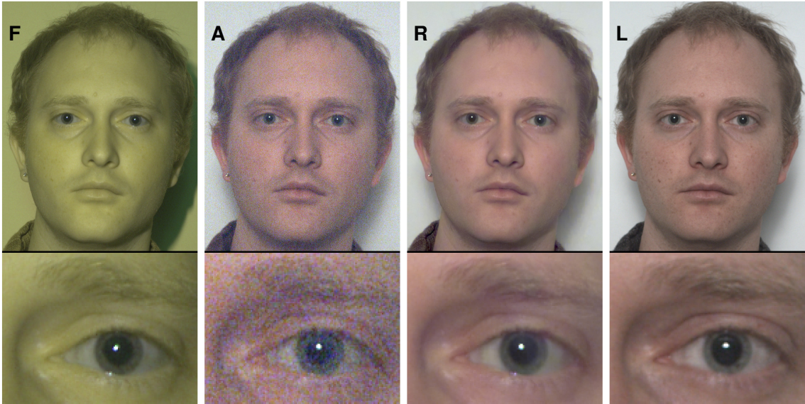
Figure 3.1: Our camera and flash system offers dazzle-free photography by hiding the flash in the non-visible spectrum. A pair of images are captured at a blur-free shutter speed, one using a multi-spectral flash (F), the other using ambient illumination (A) which in this case is 1/100th of that required for a correct exposure. The pair are combined to give an output image (R) which is of comparable quality to a reference long exposure shot (L). The figures in this paper are best viewed on screen, rather than in print.
