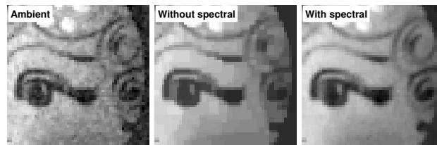
Figure 3.18: Close up of scene in Figure 3.8 illuminated by candlelight. Left: Blue channel of white-balanced ambient shot, showing high noise due to lack of blue wavelengths in candlelight. Middle: Denoising of ambient using likelihood and spatial priors only. Right: Denoising of ambient using spectral constraints from the red and green channels, in addition to the likelihood and spatial priors. The spectral constraints significantly improve performance.
