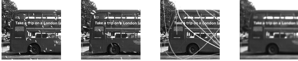
Figure 6.1: Examples of corruptions. L to R: “Snow,” “Mixed Snow,” “Scratches” and “ 7 \times 7 Blur”
