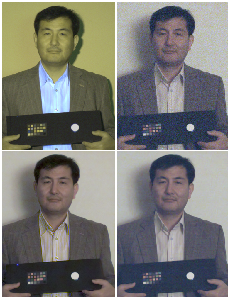
Figure 3.10: Denoising at extremely low light levels (0.9 Lux). Top-left: Flash shot; Top-right: Ambient; Bottom-left: Our reconstruction; Bottom-right: Best reconstruction of BM3D [40].
