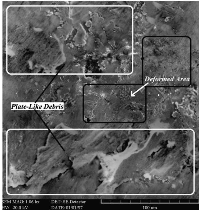
Fig. 18. SEM image of Cu-1G worn surface.
