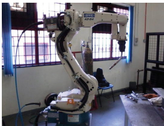
Figure 1. The OTC Almega AII-B4 articulated robot welding
