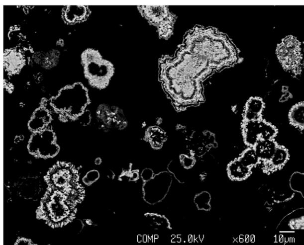
**Fig. 1.** Backscattered electron image (COMP, compositional contrast) of a polished block of the ITO powder. The image shows ITO particles (bright) embedded in epoxy resin (dark) and polished to a flat surface. Particle outlines represent transects through individual particles. Particles are generally rounded aggregates of hollow spheres with high surface to volume ratios. The scale bar is 10  $\mu\text{m}$ .
