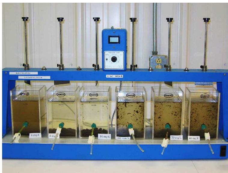
Fig. 1. Phipps & Bird Six-paddle stirrer with illuminated base.
