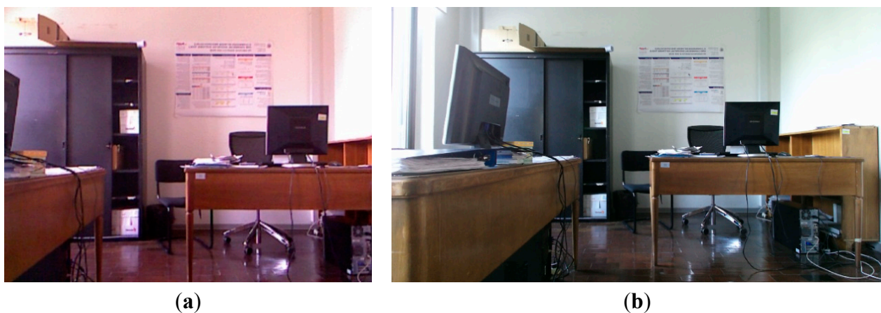
Figure 1. Kinect 1.0 RGB image (a) compared with Kinect 2.0 RGB image; (b) The two images have been acquired from the same standpoint.
