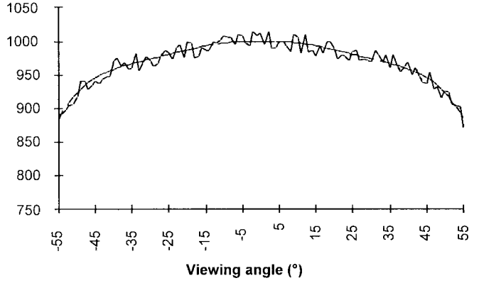
Fig. 10. Typical response on a radial section of the CCD ( p^k \cdot gm f_{lp}^k \cdot gh f_{lp}^k ). The smooth line represents the low-frequency variation of multiangular calibration p^k .
