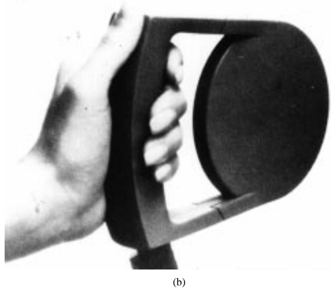
Fig. 8. Inductive charging. (a) Functional block diagram. (b) Inductive coupler.
