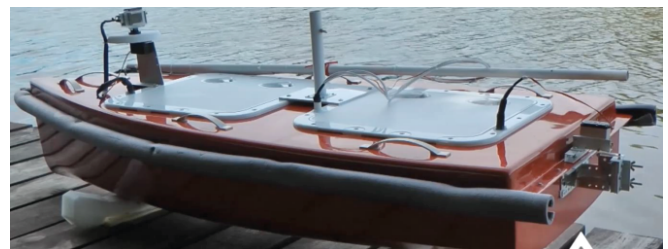
Fig. 12. UPP-1E universal measuring floating platform
