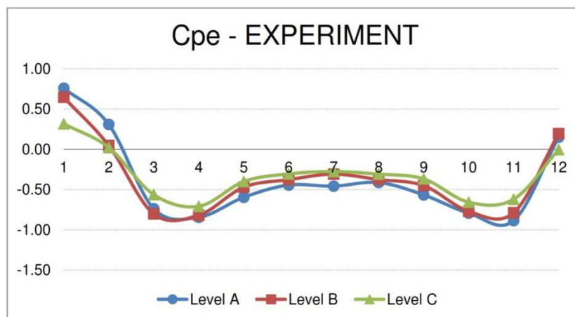
Fig. 4: Values of c_{pe} for model from experimental measurements (Level A, B, and C).
