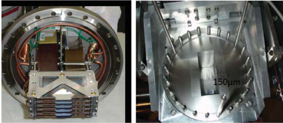
Fig. 9.4: Si detector package composed of 10 Si planes (left). Roman Pot, to separate the Si detector from the LHC vacuum via a thin window of 150\mu\text{m} thickness (right).
