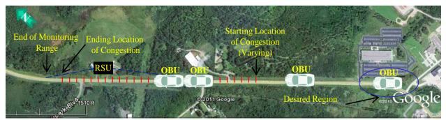
Figure 4-2: The Field Demonstration Site Showing Placement of DSRC Units and the Coverage Range of V2V-Assisted VI Traffic System.
