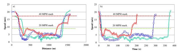
Figure 4-4: The Vehicle Speed Through the Congestion vs. Relative Distance and Time for Different Congestion Behaviors. Different Colors are for Different Test Trials.
