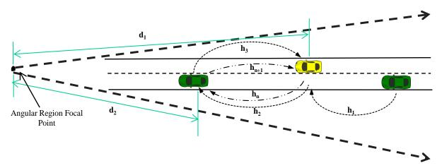
Figure 3-4: Conceptual Diagram Showing Handling of Message Back Propagation in V2V-Assisted V2I Communication Protocol.
