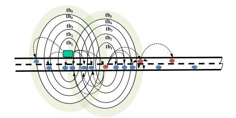
Figure 3-2: Selective Relay Functionality of V2V-Assisted V2I Communication Protocol.
