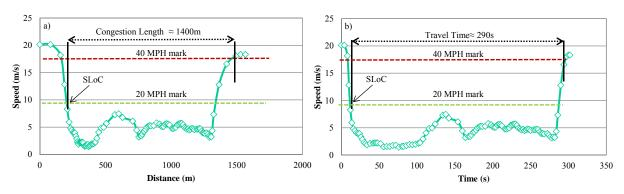
Figure 4-3: (a) The Vehicle Speed Through the Congestion vs. Relative Distance. (b) The Same Speed vs. Time.
