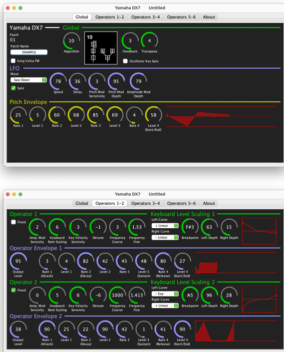
Figure 1: Edisyn’s Yamaha DX7 patch editor, showing the “Global” and “Operators 1–2” panes.
