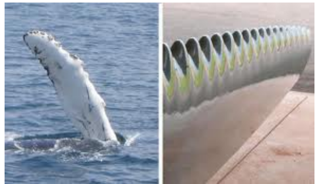
Figure 1: Design of windmill turbine blades to increase efficiency inspired by the tubercles on humpback whale flippers. (The Biomimicry Institute 2011)
