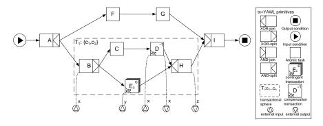
Fig. 1. Transactional workflow with sub-transactions and constraints
