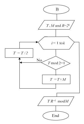
Figure 1: Algorithm of computation the Montgomery reduction for radix 2.
