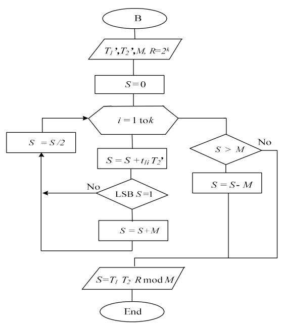
**Figure 2:** Algorithm of Computation the Montgomery modular multiplication, where  $T1' = (t1(k-1) \dots t1i \dots t12 t11 t10)$ , LSB S is last significant bit of S.
