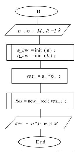
Figure 3: The scheme for computation the Montgomery modular multiplication.
