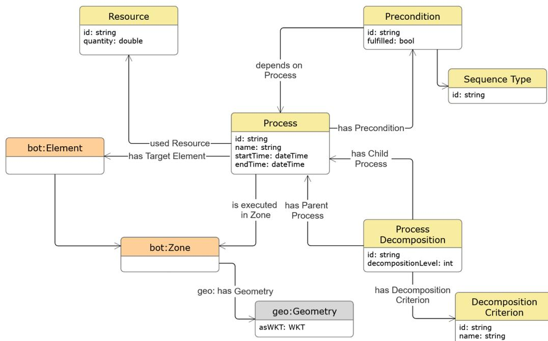
**Figure 5:** UML diagram of the Construction Scheduling Ontology (yellow: new classes, orange: existing classes, gray: optional classes).
