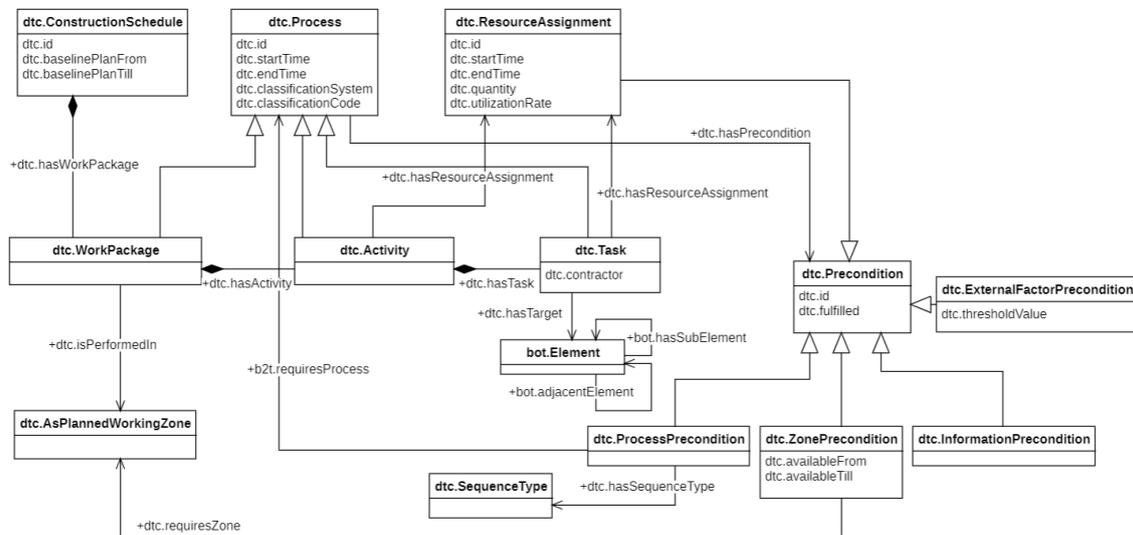
**Figure 4:** Representation of processes according to DTC [8].
