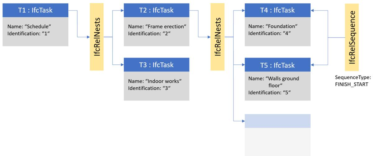
**Figure 2:** Representation of construction processes according to IFC [5].
