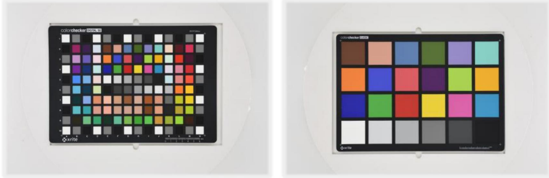
Figure 2: Captured images of the ColorChecker SG140 color chart (left) and ColorChecker 24 color chart (right) under setting exposure 1/25s and ISO 100.
