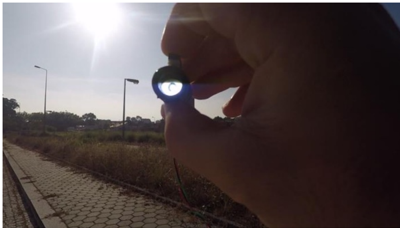
Figure 2: Example of a flash light fired in front of the camera, to assess GPS time of a frame.
