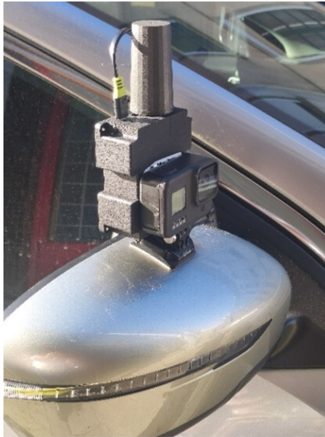
Figure 1: Gopro camera and Septentrio Mosaic Go X5 GNSS receiver, mounted in a block on a side rear view mirror of a car.
