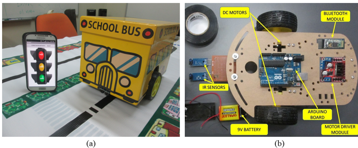
Figure 2: Development of the line-following robot (a) Traffic light app and robot design (b) Electronic and mechanical parts of the robot.
