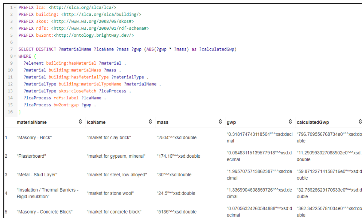
Figure 4: SPARQL (SQ1) calculating an element's GWP with results in kg CO 2eq
