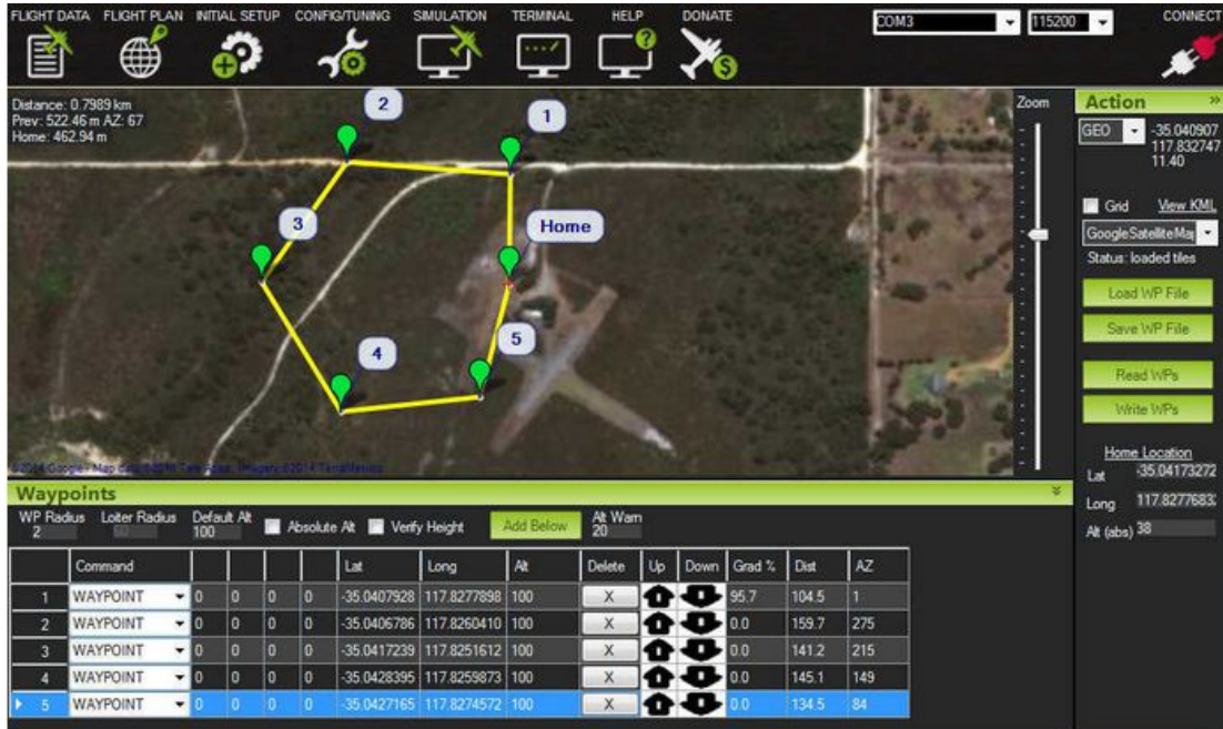
Figure 1: Setting waypoints on the example of Mission Planner in ArduPilot
