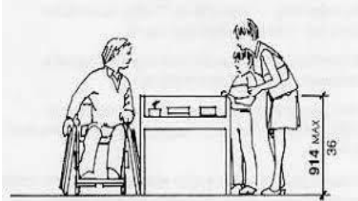
Figure 2.1: Height of free-standing display case [14].
