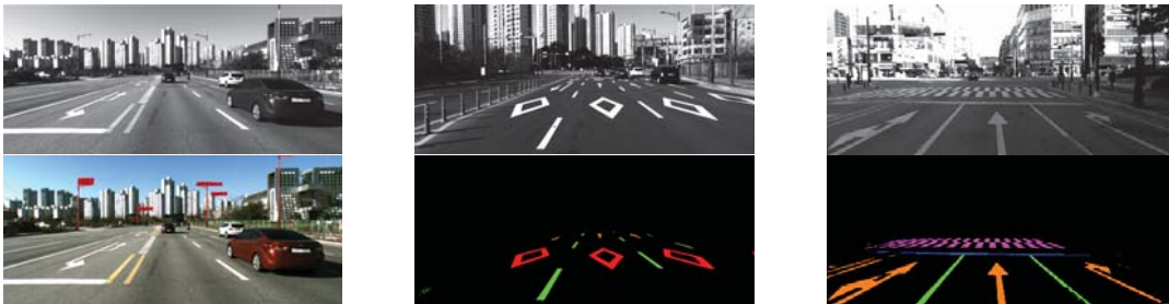
Figure 6: Feature extraction. From left to right, the feature extraction results are shown at frames 57, 303 and 356, including rod features, slowdowns and broken lines of the pavement and crosswalks, arrows and stop lines of the pavement, respectively.
