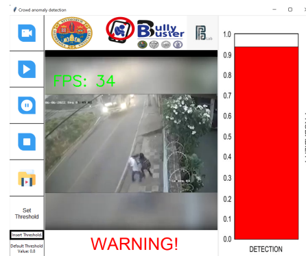
Figure 4: Demonstrator of the crowd analyzer built into the BullyBuster framework. The system detects suspicious behaviour and reports it to a human operator.
