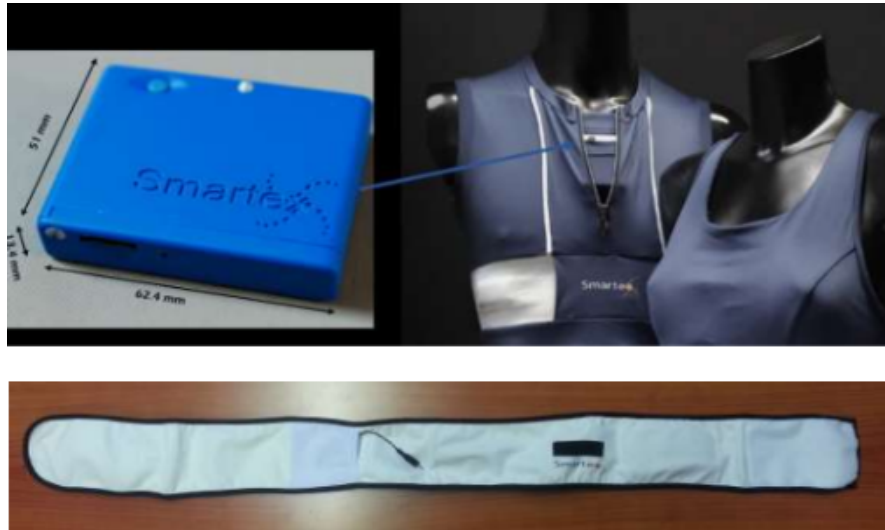
Figure 2: Smartex WWS for monitoring heart and respiratory rate.
