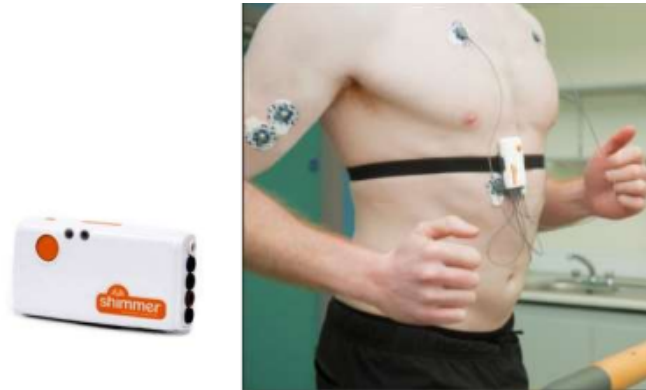
Figure 3: Shimmer cardio kit for monitoring heart and respiratory rate.
