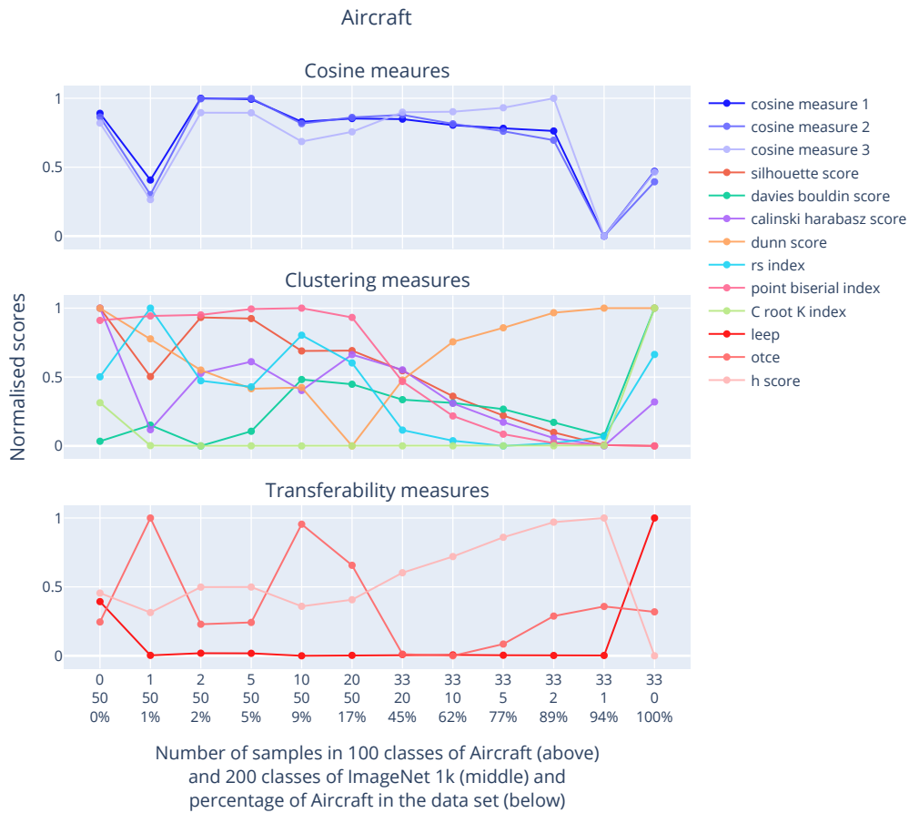
Figure 2: Scores as domain shifts from ImageNet 1k to Aircraft. Only 200 randomly selected classes of ImageNet 1k were used. Percentages are aircraft as a portion of the whole dataset
