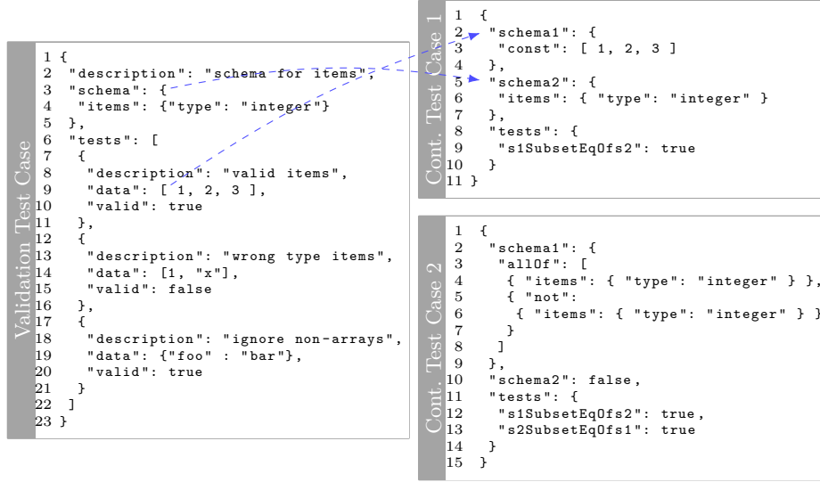
Fig. 2. Left: Test case from the JSON Schema Test Suite [12] for testing JSON Schema validators (for Draft 6, adapted from file items.json , commit hash #fe94275 ). Right: Derived test cases for JSON Schema containment. Dashed arrows indicate data flow.
