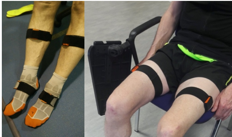
Fig. 1. Xsens inertial capture system showing sensor positions for foot, lower and upper limb.
