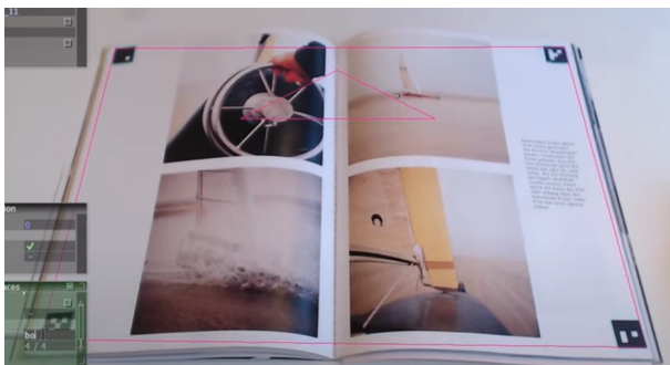
Figure 2: Object tracking using markers. They are positioned in the four corners identifying the area of interest.
