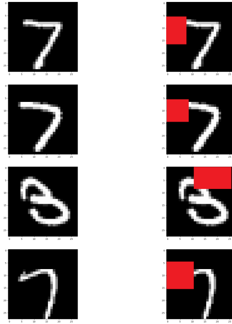
Figure 3: Original pictures and proven rectangles where we can change everything without having an adversarial example.
