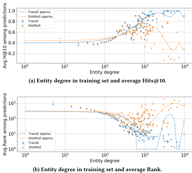
Figure 2: Training entity degree vs average performances when predicting an entity with that degree (FB15K). Dashed lines have been obtained by fitting a polynomial function of degree 4 with the least Squares technique.
