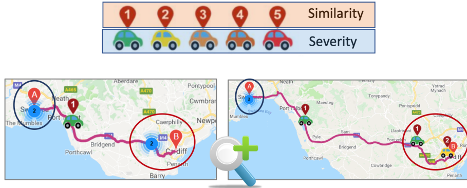
Fig. 7. Graphical explanation of the incidents found in the route. (TOP) Incident representation: numerical markers show the similarity whereas the colour of the icon reflects the severity of the incident. (BOTTOM) Incidents are grouped to simplify its visualization and detailed when zooming in.
