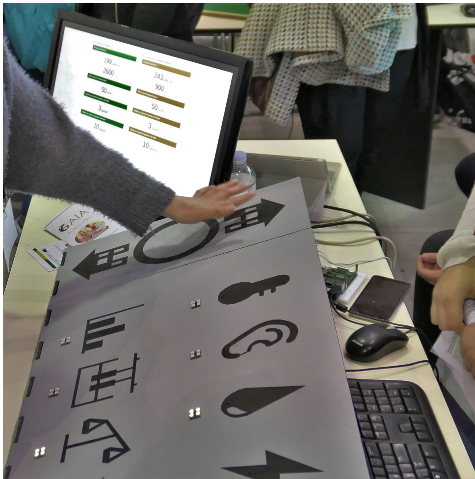
Figure 5: An example of the more “creative” uses of school building datasets. Here, an interactive installation acting as a “control panel” that can be installed at a school corridor, allowing students to “play” with real-time data and statistics related to energy consumption and environmental parameters.
