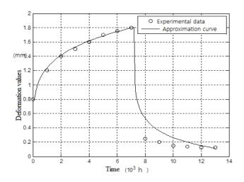
Fig. 1. Identification of the fractal parameters for Maxwell's model
