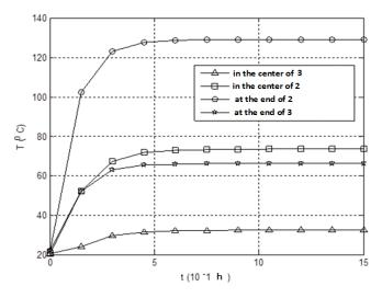
Fig. 2. Temperature change at different geometric points of biomaterial samples with different densities, taking into account fractal parameters.
