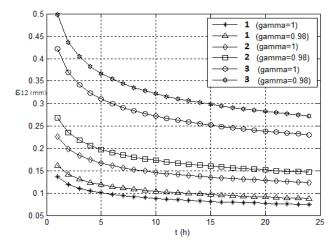
Fig. 3. Change in the deformation component  $\mathcal{E}_{12}$  depending on the type of biomaterial
