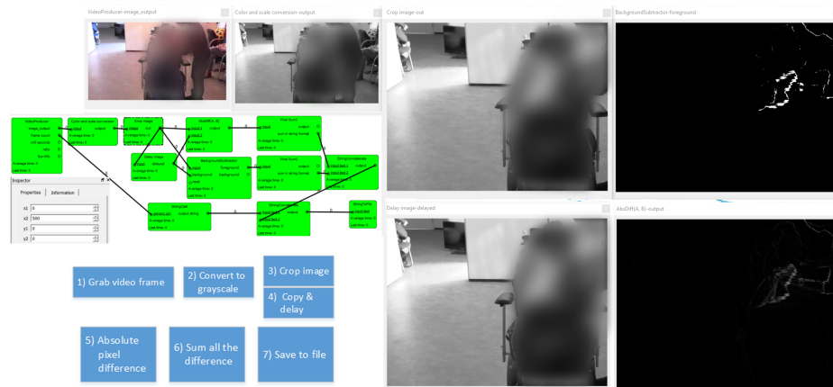
Fig. 2. An example of the process of Simplified Motion Energy Analysis, where we can see the movement of a caregiver on the right. The blocks from the ParleVision pipeline (green) perform similar steps as written out in the blue blocks.
