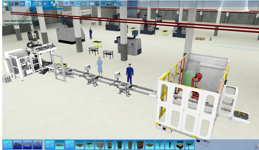
Figure 1. GIOVE-VF: example of factory layout including a production line that consists of five workstations
